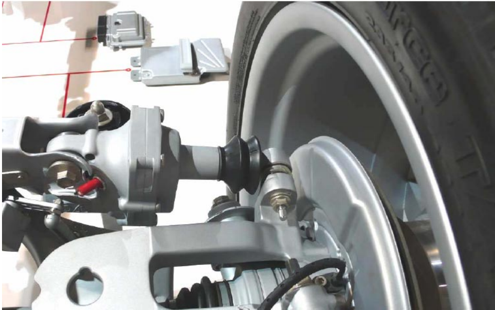
Fig. 3: Electro-mechanical Conceptual Prototype in Rear Axle Assembly
